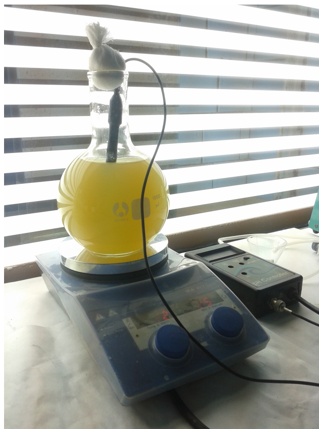
Fig. 1. C. closterium cultivation on a nutrient medium with sodium bicarbonate as the sole carbon source
