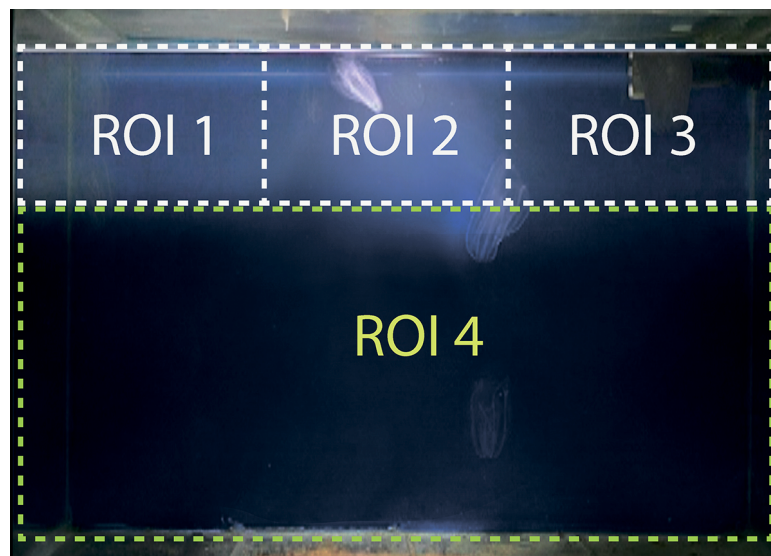
Fig. 2. Regions of interest (ROI): 1, a region with high level of illumination; 2, with medium level of illumination; 3, with low level of illumination; 4, a dark region
